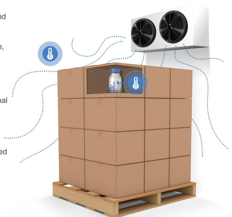
**Fluctuations in ambient air can affect quality and cause food safety issues, however, changes are sometimes minimal and have insignificant effect on product temperature. The only way to be certain is by using product emulation, in order to have a complete history of internal temperature readings throughout the cold chain.**
